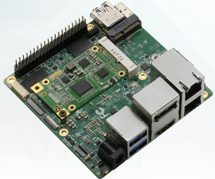
The AI Core X mPCIe module features the Intel Movidius Myriad X, a low-power high-performance VPU designed for AI acceleration with Edge Computing. The Intel Movidius Myriad X offers speeds up to 105 fps (80 typical) and over 1 trillion floating point operations as a dedicated neural network accelerator. The AI Core X is compatible with the Intel distribution of OpenVINO Toolkit, and supports TensorFlow and Caffe frameworks.
