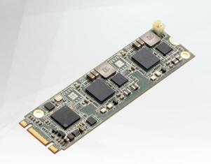
The AI Core XM2280 m.2 module features two Intel® Movidius® Myriad™ X VPUS, a low-power highperformance accelerator designed for Al Edge Computing. The AI Core XM2280 delivers speeds up to 200 fps (160 typical) and over 2 trillion floating point operations as a dedicated neural network accelerator.
