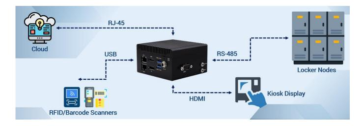
The key thing that set the <u>UP Squared 7100 Edge</u> apart from other choices was its multifaceted and broad selection of interfaces, especially given its small size. The customer's existing smart locker infrastructure relied on RS-485 serial communication via COM port, and so the task of controlling the application's locker hardware leveraged the UP Squared 7100 Edge's dual COM ports.
