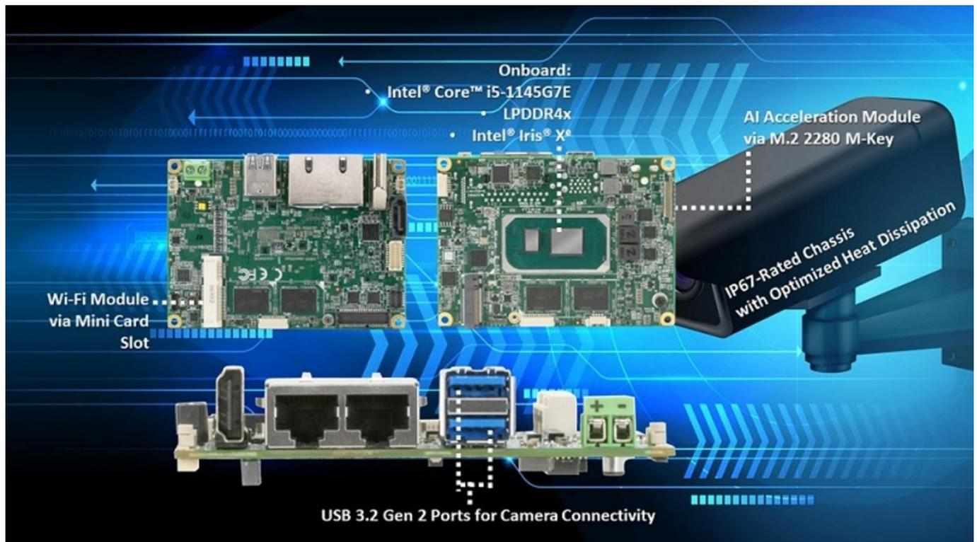
Enclosed within the company's hermetically sealed, IP67-rated chassis, the [PICO-TGU4](#) was equipped with the necessary functions to ensure the unit could be deployed across a wide spectrum of security applications. These applications included perimeter monitoring, maritime surveying, highway traffic control, and border surveillance.
