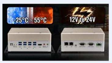
Measuring in at just 180mm x 136mm x 78mm, the system is compact, making it suitable for integration into the store's self-checkout kiosks. In terms of durability, the <a href="BOXER-8642AI">BOXER-8642AI</a> was suitable by design, with the primary concern of fluctuating power supply negated by the system's broad 12V to 24V DC power input range.
