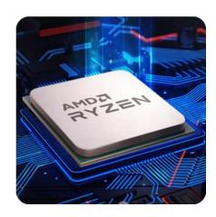
With up to 8 cores and 16 threads of processing power, sophisticated Zen 2 x86 core architecture, and 7nm process technology, the PICO-V2K4's AMD Ryzen™ V2000 series CPU provided the application with a unique leap in both performance and power-efficiency, particularly on the PICO-ITX form factor.
