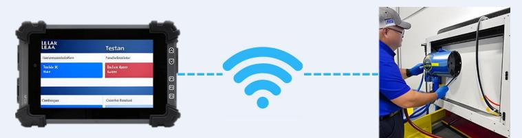
The customer's solution comprised a leak detection unit and a remote controller. The unit consisted of a vacuum pump, chamber, and sniffing inlet port, while the <u>RTC-</u><u>710RK</u> was deployed as the remote controller with a customized flex mount for easy storage and access during use.
