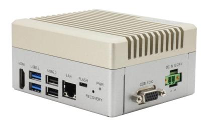
Measuring just 105mm x 90mm x 52mm and weighing only 2.4 lb. (1.1Kg), the BOXER-8651AI is the market's smallest fanless system equipped with an integrated NVIDIA® Jetson Orin™ NX module.
