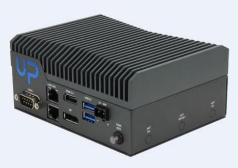
Given the <u>UP Squared Pro 710H</u> <u>Edge</u> is both compact, measuring just 5.28" x 4.13" x 2.36", and lightweight, at 1.8 lb., it was easily installed via wall mount at the entrance of a number of department stores. Equipped with two USB Type-A and two 2.5GbE ports, AAEON's customer had a variety of interfaces through which cameras could be installed on the device. They opted for high-
