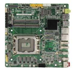
Given the technical needs of the project, particularly with respect to handling high volumes of data and subsequent storage needs, the AAEON team recommended the MIX-Q670D1, a Mini-ITX motherboard equipped with the Intel® Core™ i7 processor 14700.
