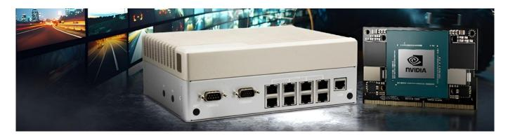
The <u>BOXER-8658AI's</u> unique selection of interfaces was a major factor in its selection for the project. With the PC able to support eight PoE cameras via RJ-45 ports, the client's security system could maintain comprehensive surveillance of the vehicle's surroundings.
