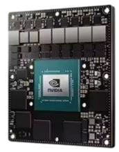
By choosing AAEON's <u>BOXER-8645AI</u>, the client also leveraged exceptional AI inferencing, given the PC's NVIDIA® Jetson AGX Orin™ platform. Relying on the 2048-core NVIDIA Ampere architecture GPU with 64 Tensor Cores and up to 275 TOPs of AI performance, the <u>BOXER-8645AI</u> provided the vehicle with the tools needed to detect and recognize its
