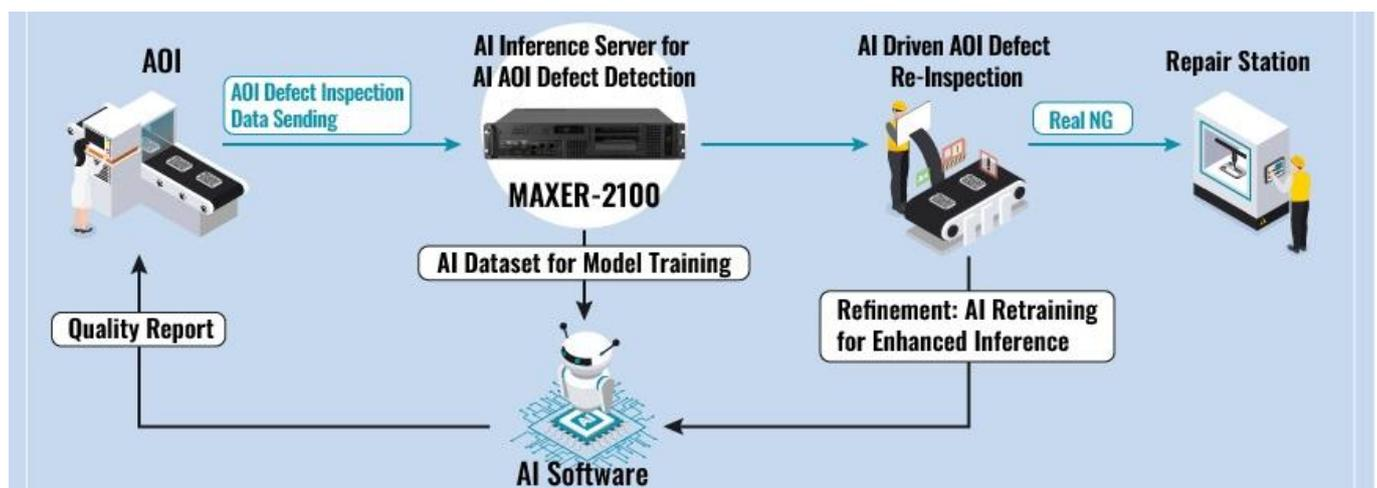
The Hawkeye solution acquired images of components, solder joints, traces, and other features of the PCBs via an AOI device.
