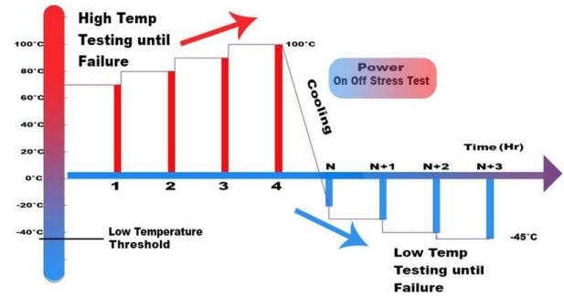
**Figure 5 - AAEON Board Stress Test**
