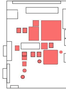
**Figure 2 - Poor Thermal Component Design**
