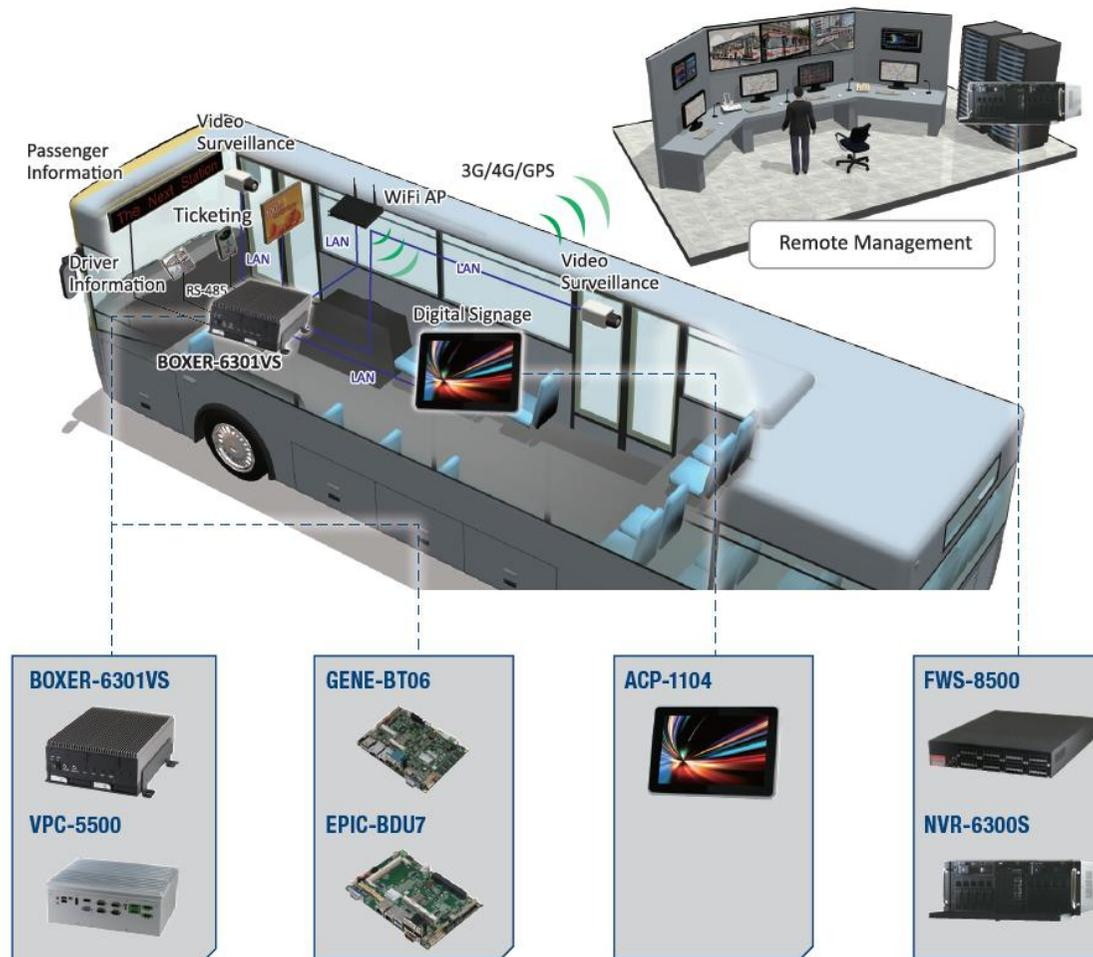
With AAEON's fan-less BOXER-6301VS Embedded Box PC and VPC-5500 Vehicle PC, passengers may enjoy network connectivity via in-vehicle WiFi, while infotainment content plays on the onboard displays. The driver can monitor the conditions in and around the bus on a screen displaying the feeds from onboard cameras.
