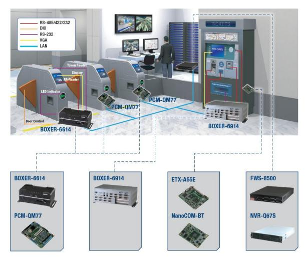
Access control or paid access often involves the use of a turnstile, a unidirectional gate which grants entry to a single person at any one time. While turnstiles of the past served the sole purpose of regulating the flow of people, their modern iterations are basically computers of their own that are an integral part of the business.
