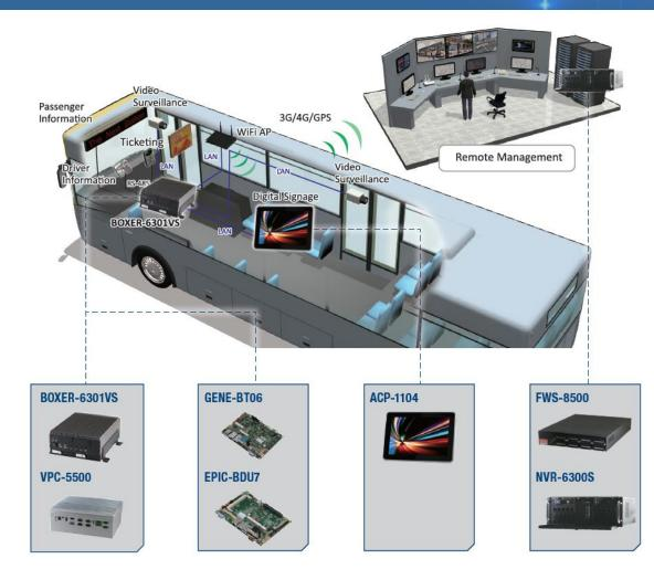
With AAEON's fan-less BOXER-6301VS Embedded Box PC and VPC-5500 Vehicle PC, passengers may enjoy network connectivity via in-vehicle WiFi, while infotainment content plays on the onboard displays. The driver can monitor the conditions in and around the bus on a screen displaying the feeds from onboard cameras.
