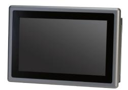
Except the difference in dimensions (10.1" for ACP-1106 and 7" for ACP-1076), both new panel PCs share many similar features like two 10/100/1000 BASE-TX RJ-45 ports, 1 x mSATA socket, 1 x mini-card socket, projected capacitive multi-touch, IP65 aluminum front bezel, fanless design, VESA mount option and DC 9-30V power.
