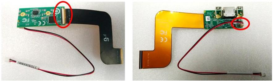
**Step 4:** Unlock the main board FPC connector, then plug the FPC cable and power cable into it.
