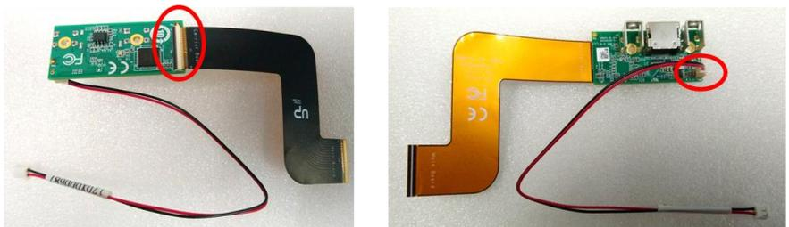
**Step 3:** Unlock the main board FPC connector, the plug the FPC cable and power cable into it.
