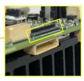
**Step 3**: Plug the FPC cable into the FPC connector, noting the direction of the FPC cable via the printing on its top side, as shown.
