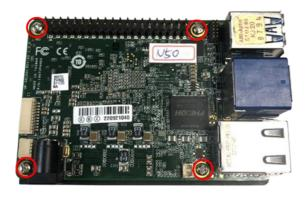
**Step 2:** Lock the four pillars and ensure the USB wafer connection on the motherboard is accessible.
