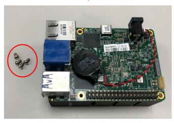
Step 2: Lock the four pillars and make sure to unlock the UP 4000's FPC connector.
