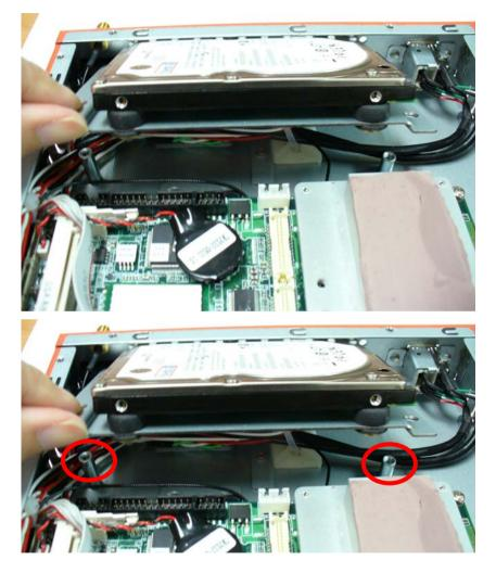
Step 4: Screwing the HDD bracket up and connecting the HDD cables with the main board.
