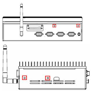
Step 3: Fasten the four HDD screws and black damper and then you can put the HDD in it.
