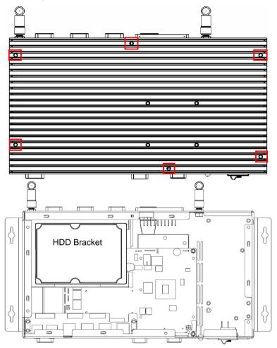
Step 2: Unfasten the two screws on the front side and right side of the chassis.
