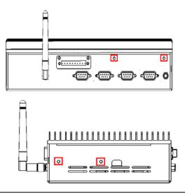
Step 6: Fasten the screws on the top of the heatsink.
