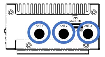
Step 3: Install the RF coaxial cables on the antenna holes.
