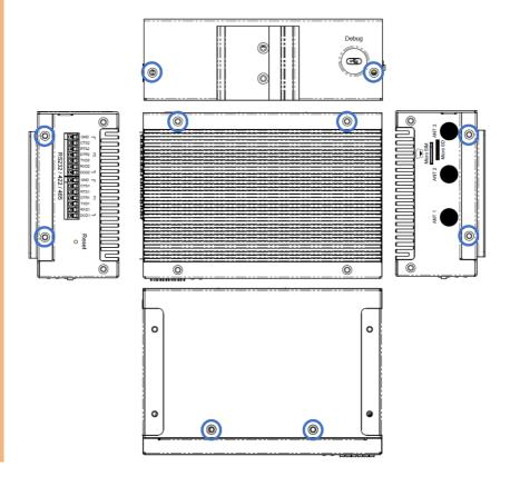
Step 2: Remove the plugs from the antenna holes:
