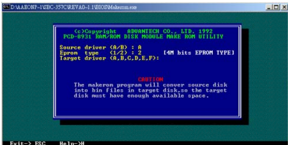
Pic3 Select "2" in "Epron type" for SBC-357 Rev.C is with 4M bits (512 Kbytes) on board. And then choose the target disk drive to save the ROM files.
