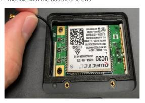
6. Attach the antenna cable to the MAIN connector of the LTE module
