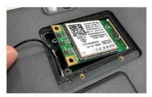
5. Secure the LTE module with the attached screws
