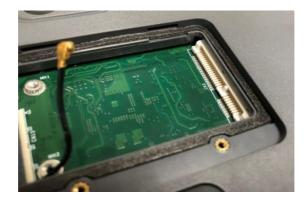
4. Slide the LTE module into the socket
