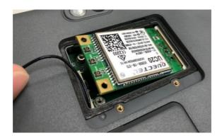
5. Secure the LTE module with the attached screws
