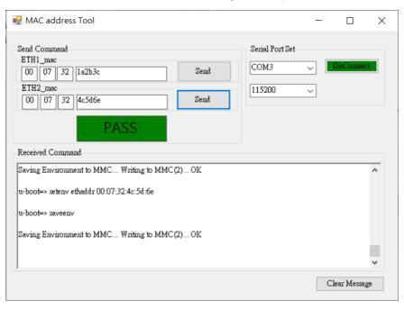
You can also verify the MAC address in the system using the ifconfig command. For the mainboard, check eth1, and for the PER-T650, check eth0.
