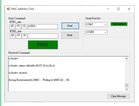
You can write another MX8P without disconnecting the serial port.
