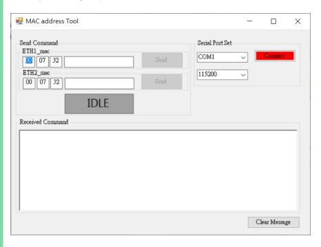
**Step 4:** Enter the MAC address: use ETH1 for the mainboard and ETH2 for the PER-T650.
