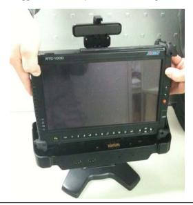
Step 5: Press the lock to lock the Rugged Tablet Computer and finish the installation
