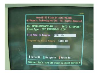
The board will restart when it is finished refreshing the BIOS. The display will show a LVDS message as seen below on the first POST screen.
