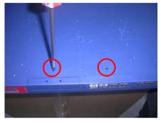
Step 2: Remove the null Module cover or existing LAN module
