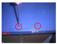
Step 2: Remove the null Module cover or LAN module
