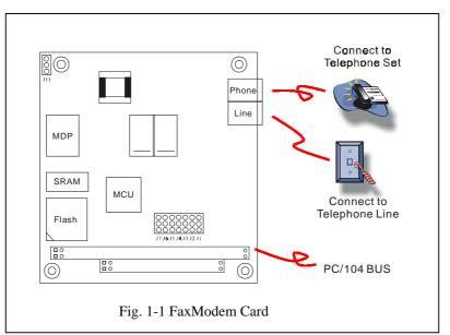
Phone: Accepts a Telephone set Connected Parallel to your Modem.
