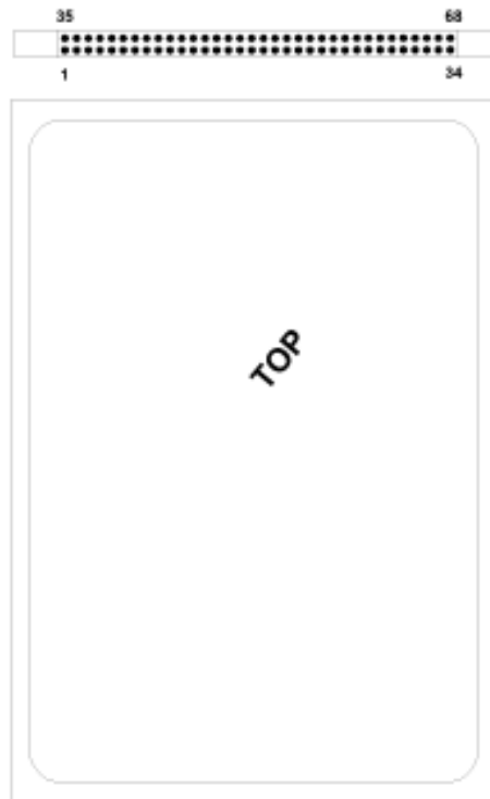
PCMCIA card showing pin assignments
