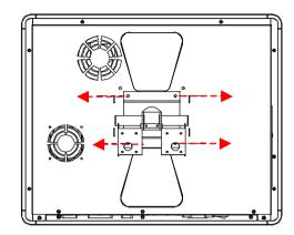
2. Unscrew the ten attachment screws used to hold the rear maintenance cover.
