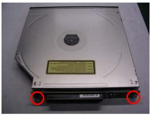
5. Fasten screws on bracket to adhere to the CD-ROM
