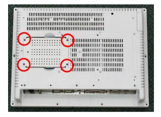
Get the 2.5" HDD ready and fasten the four screws on HDD and put the rubbers on screws
