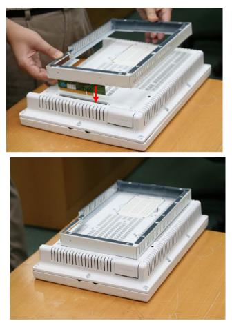
4. Fix the rack with the screws on the corners.
