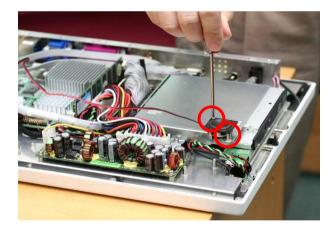
10. Lock the plastic cover of the ONYX-150 and complete the installation
