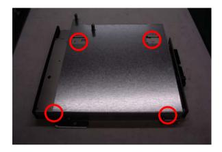
Insert IDE Cable into CD-ROM Module, fix CD-ROM Module into ONYX-150 and fasten the three screws
