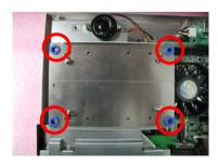
4. Assemble 2.5"HDD into disk module.
