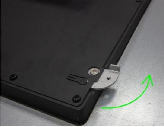
**Step 3-** Use screws to secure the panel onto the wall with the wallmount brackets
