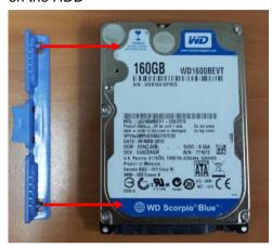
Step 2: Align one mounting hole on the right side to gauge bracket pin by sloping
