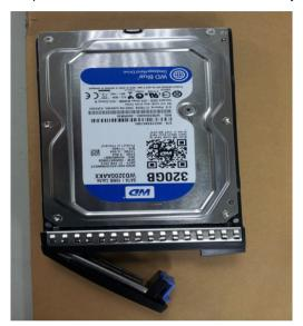
Step2: Fasten the two screws on the both sides to fix the HDD tray
