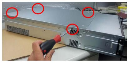
Step 2: Thumb finger touch downward and then push back the rear back cover
