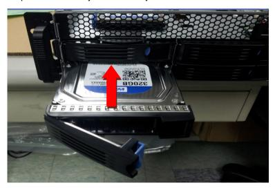
Step 4: Push the leaver to latch HDD tray
