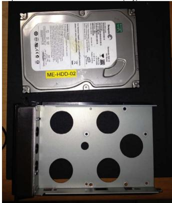
Step 3: Fasten the HDD on the bottom bracket with three screws
