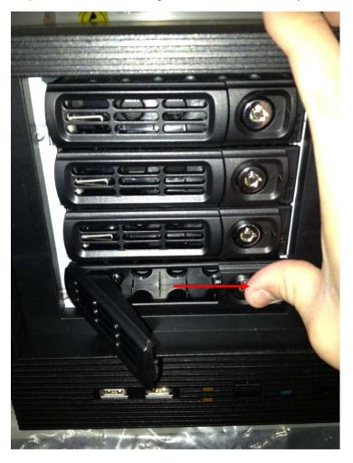
Step 2: Put the HDD to the HDD bracket (tray)
