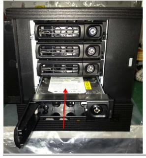
Step 5: Push the HDD tray to the chassis until it has been firmly locked
