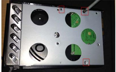
Step 4: Insert the HDD tray back to the chassis
