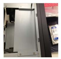
Step 2: Shift the HDD upper bracket from right to left and remove it.
