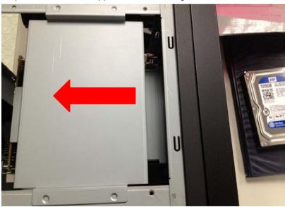
Step 3: Put the hard disk into the drive bay and lock it with four screws
