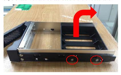
Step 4: Fasten the 2 screws on each side of the HDD.
