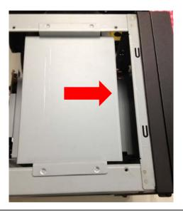
Step 5: Firmly lock the HDD bracket with 4 screws.
