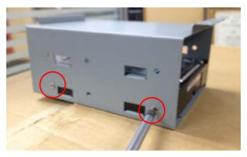
Step 4: Put back the HDD bracket and push it to the right until it's locked in position.
