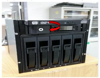
Step 6: use a magnetic screwdriver to secure three screws the optical drive
