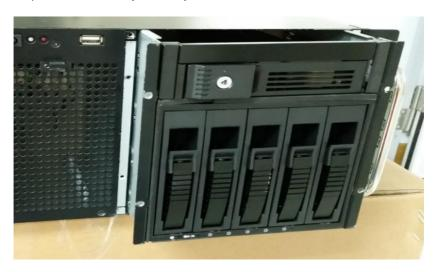
Step 4: Remove the slim optical drive bay by pressing buttons on both sides
