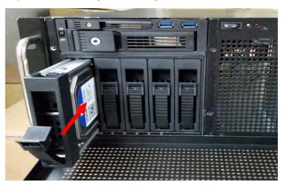
Step 4: Push the lever to latch the HDD tray
