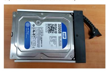
Step 2: Fasten the four screws to secure the HDD with the HDD tray
