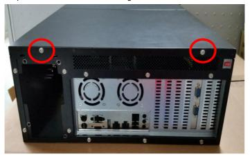
Step 2: Thumb finger touch downward and then push back the rear back cover
