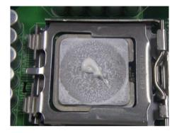
c. Place the Heatsink on the top of CPU. Please make sure that the four screws are aligned with the holes on the board.
