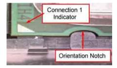
Step 3: (Positioning the CPU into socket)
