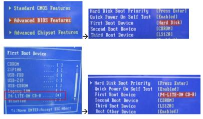
Above is using IDE CDROM, cause ICH9 don't support IDE interface, FSB-960G using JMICROM chip as a SATA to IDE bridge, this is why when SATA mode set to Raid, you must choose P4-XXXX. If using USB CDROM you just need choose USB-CDROM.
