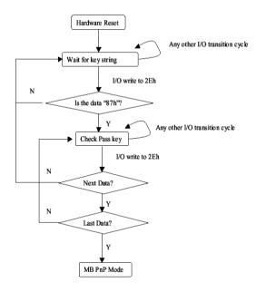
There are three steps to complete the configuration setup: (1) Enter the MB PnP Mode; (2) Modify the data of configuration registers; (3)
