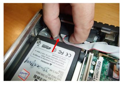
Step 9: Done installing the HDD. Close and screw the bottom case of the  ${\sf GES}\xspace{-}3300{\sf F}$
