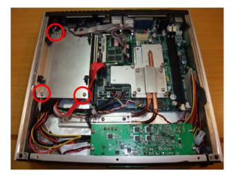
Step 3: Disconnect the SATA and Power cables (The CompactFlash card is optional. If you did not buy the CF card, you may skip the step 3 and step 4.)
