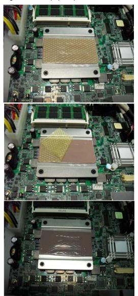
Step 4: Get the SODIMM stuck with thermal pad ready
