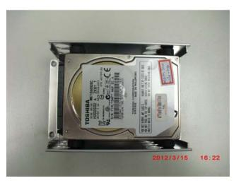
Step 3: Fasten the four screws to lock the HDD bracket and connect the SATA and power cable
