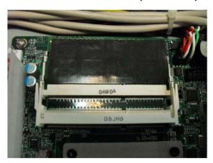
Step 6: Install the second SODIMM to the upper layer of memory slot
