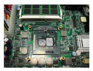
Step 2: Cover the CPU bracket and fasten the four screws to fix the CPU bracket, and then stick the thermal pad on the bracket
