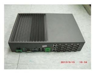
Step 8: Fasten the screws on the right and left cases of GCS-2500 and you've done installing the CPU and RAM module
