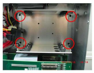
Step 2: Place the HDD to the HDD bracket
