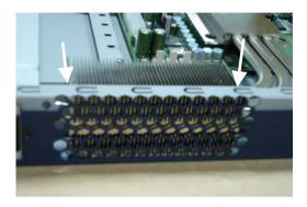
Step 12: Fasten the four screws of the heatpipe
