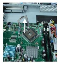
Step 7: Lock the CPU Socket
