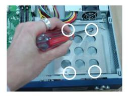
Step 2: Lift up the Hard Disk Drive Bracket aside
