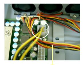
Power cables of FAN Module are under the 12V Power Cable
