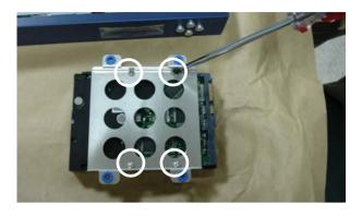
Step 4: Overturn the Hard Disk Drive and put it into the chassis
