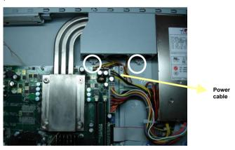
Step 15: Insert the Power cable of Fan Module
