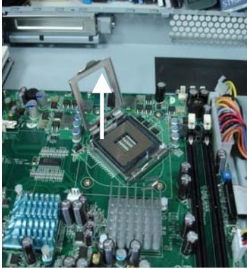
Step 7: Lock the CPU Socket
