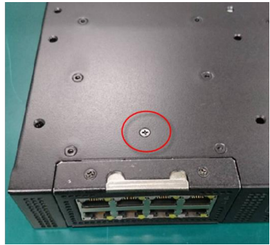
Replacing NIM Module
